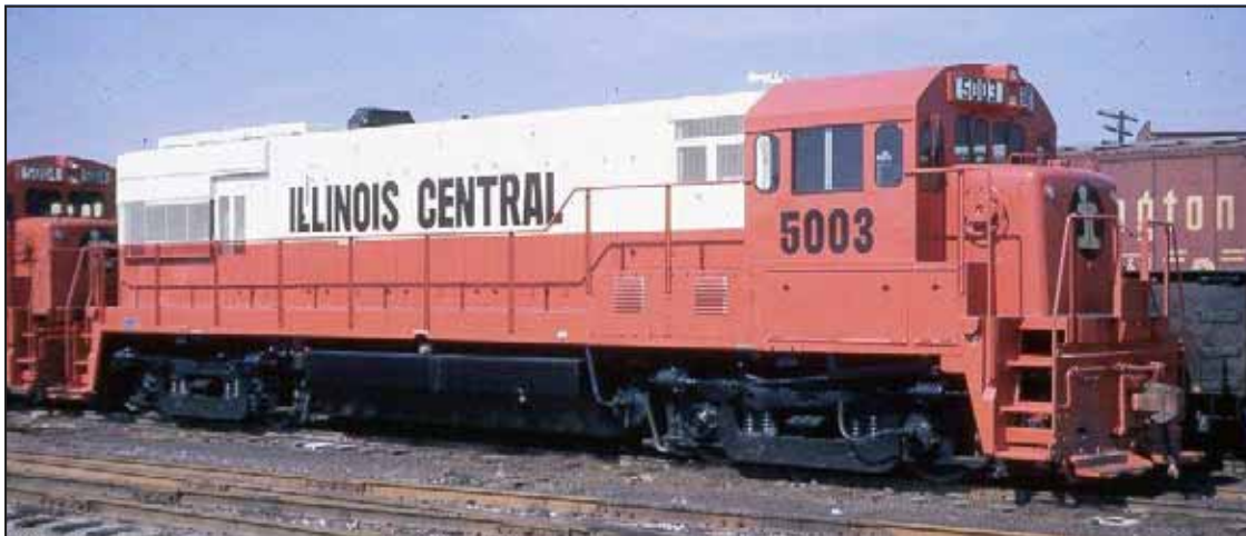
Illinois Central U30B 5003. This locomotive was photographed shortly after delivery by General Electric, as the exhaust stack is still covered with black plastic. The photograph was taken at Louisville, KY in March of 1967. Tom Smart, collection of J LHunt.
